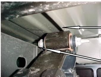
NOTE: THIS PINCH WELD MUST BE BENT UP OUT OF THE WAY IN ORDER TO BE ABLE TO REMOVE THE STOCK UPPER LEAF SPRING EYE TO SHACKLE BOLT.
