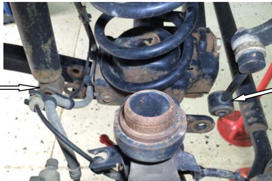
LOWER SWAY BAR CONNECTING LINK REMOVED FROM AXLE
