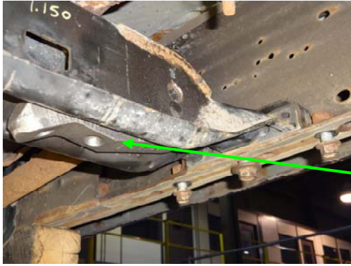
NEW RE-INDEXED TORSION BAR KEY BEING INSTALLED .
