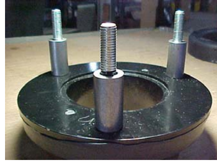
THREE STEEL SUPPORT SLEEVES BEING INSTALLED OVER THE NEW SPRING SEAT STUDS
