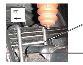
SUPPLIED WEDGE WITH THE THICK END OF THE WEDGE TOWARD THE REAR OF THE VEHICLE.
