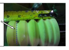
FACTORY STEEL SPACER INSTALLED WITH THE TAPER DOWN INTO THE TOP OF THE BUMPSTOP
