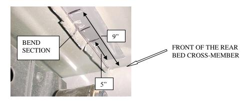
8. USING A MALLET/DUCKBILL VISE GRIPS BEND THE PINCH WELD OVER AND FLAT UP AGAINST THE BOTTOM OF THE BED. NOTE THIS IS A DOUBLE LAYER OF SHEET METAL IT WILL BE DIFFICULT TO BEND OVER, IT MAY HELP TO CUT UP THROUGH THE PINCH WELD USING A SMALL CUTOFF WHEEL. IF YOU CUT THE PINCH WELD BE CAREFUL NOT TO HIT THE BED FLOOR. REMOVE THE TAPE AND COAT ALL AREAS OF BARE METAL WITH A GOOD METAL PRIMER AND PAINT TO KEEP THE PINCH WELD FROM RUSTING.
