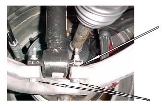
STRUT LOCATED ON TOP OF LOWER CONTROL ARM
