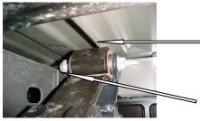
NOTE: THIS PINCH WELD MUST BE BENT UP OUT OF THE WAY IN ORDER TO BE ABLE TO REMOVE THE STOCK UPPER LEAF SPRING EYE TO SHACKLE BOLT.
