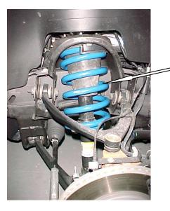
STRUT ASSEMBLY INSTALLED UP THROUGH THE LOWER AND UPPER CONTROL ARM.
