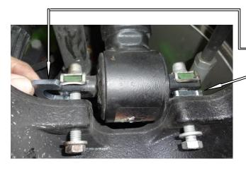
OPTIONAL STRUT SHIMS BEING INSTALLED BETWEEN THE TOP OF THE LOWER CONTROL ARM MOUNT AND THE BOTTOM OF THE STRUT MOUNT
