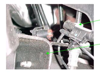
ANTILOCK WIRE CONNECTOR BEING DISCONNECTED.
