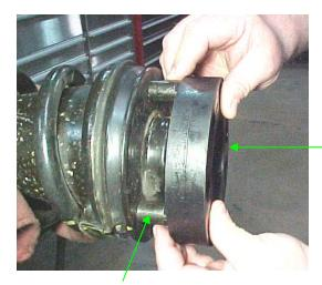
URETHANE SPACER BEING INSTALLED OVER THE STRUT EXTENDERS.
