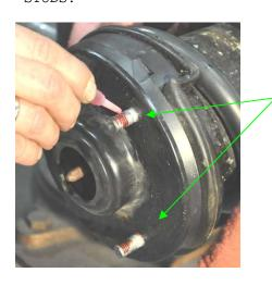
HIGH STRENGTH THREAD LOCKER BEING APPLIED TO LOCK THE NEW STRUT EXTENDERS IN PLACE.
