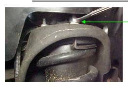
18 MM WRENCH LOOSENING THE THREE OUTER UPPER STRUT MOUNTING BOLTS.
