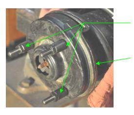
STRUT EXTENDERS BEING INSTALLED OVER THE TRIMMED STRUT UPPER MOUNTING STUDS.
