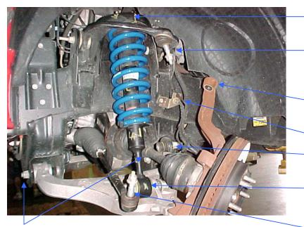
LOWER CONTROL ARM TO FRAME MOUNTING HARDWARE UPPER STRUT INDEX MARK
