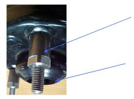
STRUT EXTENDERS BEING INSTALLED OVER THE TRIMMED STRUT UPPER MOUNTING STUDS.
