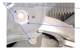
LOWER CONTROL ARM TO FRAME MOUNTING HARDWARE.
