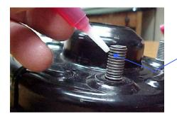
HIGH STRENGTH THREAD LOCKER BEING APPLIED TO LOCK THE NEW STRUT EXTENDERS IN PLACE.
