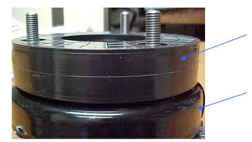
URETHANE STRUT SPACER BEING INSTALLED
